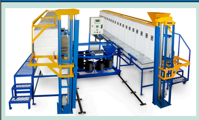
Figure 1 - 40-bin micro dosing system
