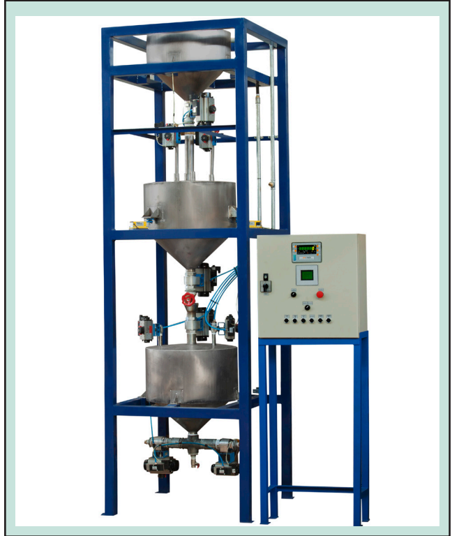
Figure 6 - oil weighing station
